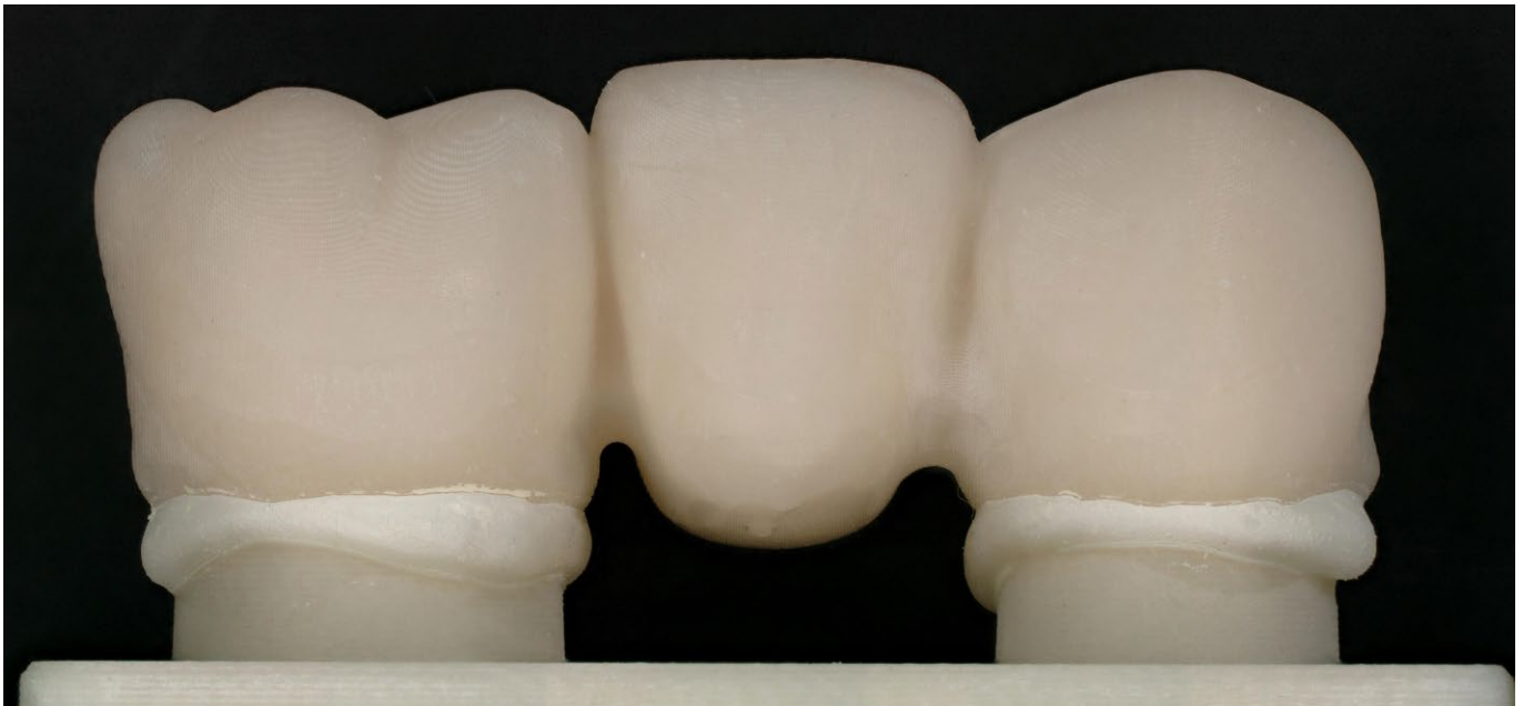
Figure 1: VarseoSmile® TriniQ® specimens for the chewing simulation and subsequent breaking load test
