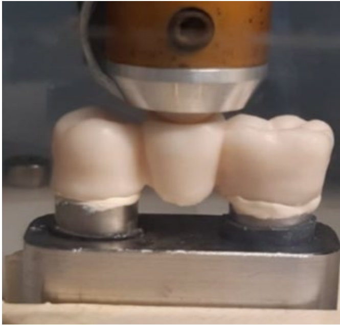
Figure 2: Test setup in the chewing simulator
